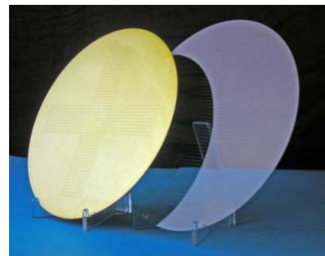
Figure 2. 8" Lens Master (left) and replicated 8" Wafer (right) [2]
